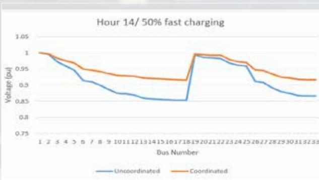
Figure 6. Voltage profile for hour 14 as fast charging
