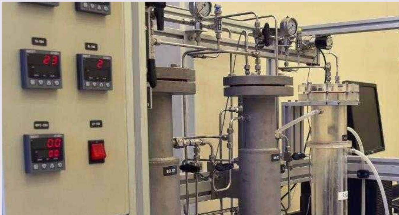
Figure 2. Inert particles spouted bed reactor system at Qatar University
