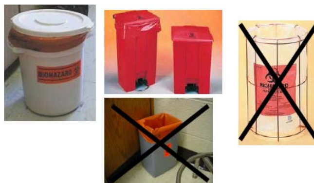
Figure 5 - Container for contaminated solids
