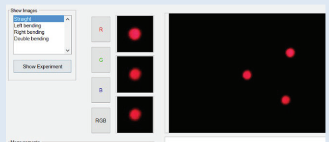
Figure 6: Graphical user interface showing the three light intensity circles are divided and compared individually to project the right shape prediction.
