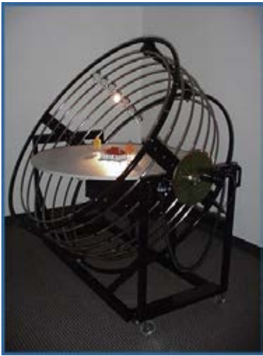
View of the Heliodon and a physical model to be tested in the Heliodon
